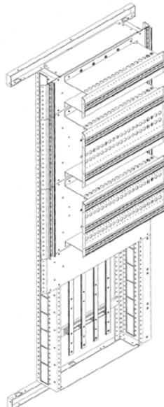
The system is designed so that the standard type (circuit breakers) can be integrated with other types (contactors) with no need to adapt other (different) structures to the primary system to support the different types.
