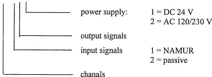
All variations are marked with :  $\text{Ex}$  II (1) GD [EEx ia] IIC/IIB and the variations type 9170/\*0-\*0-11, type 9170/\*0-\*1-11 and type 9170/\*0-\*4-11 are marked additionally with  $\text{Ex}$  II 3 G EEx nAC II T4.
